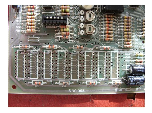
Module correctly located (pressed into DIL sockets in this case.)
