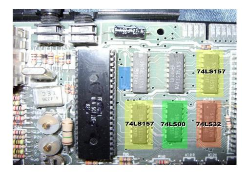
Issue 3 PCB - Jumper positions highlighted in blue (shown with heatsink removed)
